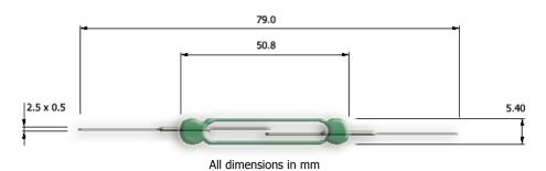
This reed switch is physically robust and can switch up to 120W. The two types of contact ratings available cover a wide range of high wattage applications. When supplied in an RAT group and used normally closed with a biased magnet, it is especially useful in elevator and hoist applications. Close differential characteristics can also be built into this reed switch. This reed switch is Lead (Pb) free and RoHS compliant.
